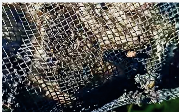
This sock shows dark areas where oils have been absorbed, as well as the light areas that show the basalt fibers can absorb much more.
